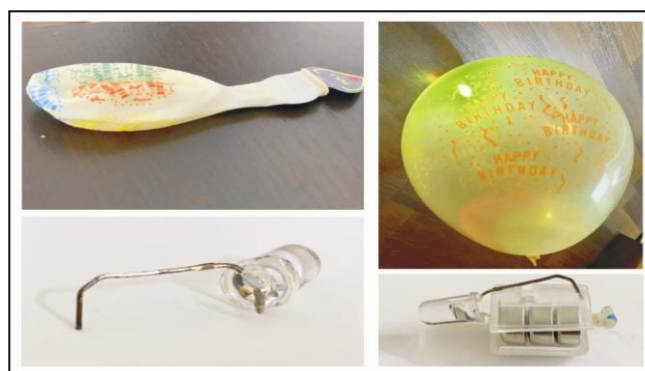
Fig. 3: LED balloon uses an encased battery attached with an LED bulb via hook.
